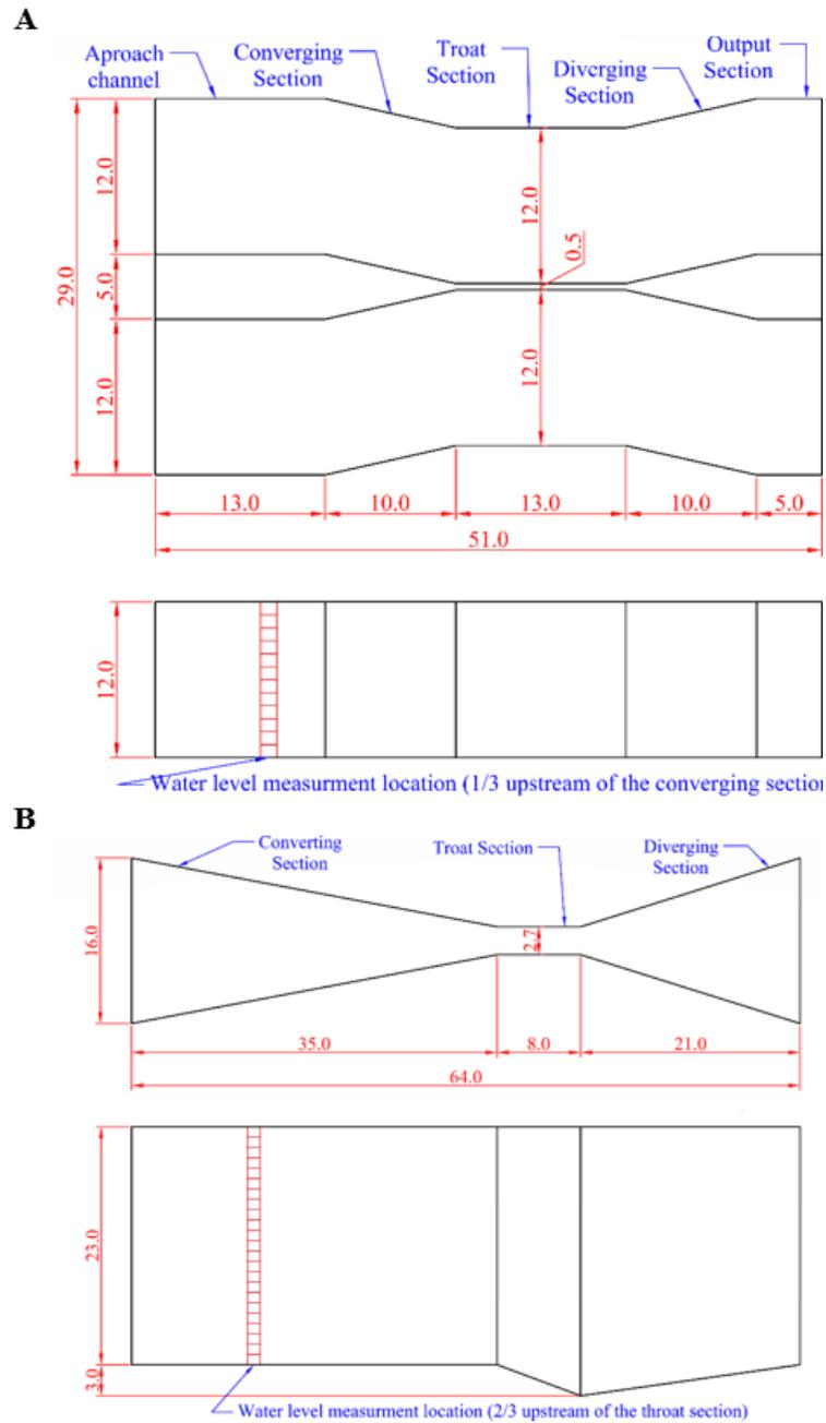
**Figure 2.** Graduated ruler on the WSC flume (A) and on the Parshall flume (B). Dourados / MS, 2019/2020.
