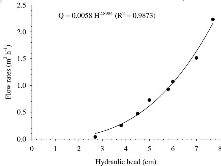
The minimum and maximum flow rates in the WSC flume were 0.039 and 2.23 m³ h⁻¹, respectively. However, in runoff work on ramps, Portocarrero, Andrade e Campos (2017) used ramps of 44 m² (11 x 4), so the flume would absorb up to a
