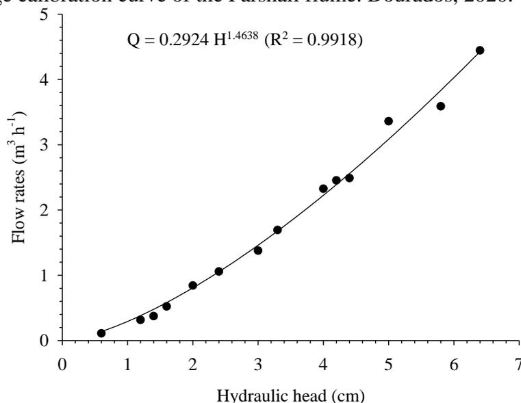
The minimum and maximum flows in this calibration correspond, respectively,  $0.11 \text{ m}^3\text{h}^{-1}$  and  $4.44 \text{ m}^3\text{h}^{-1}$ . Through the calculation of  $Q = C \cdot I \cdot A / 360$ , taking into account the same previous data of the WSC flume, with infiltration coefficient of the terrain  $C = 0.4$  (high flow), and considering a contribution area equal to  $44 \text{ m}^2$ , concludes the maximum precipitation that the system can collect is  $252.6 \text{ mm h}^{-1}$ .
