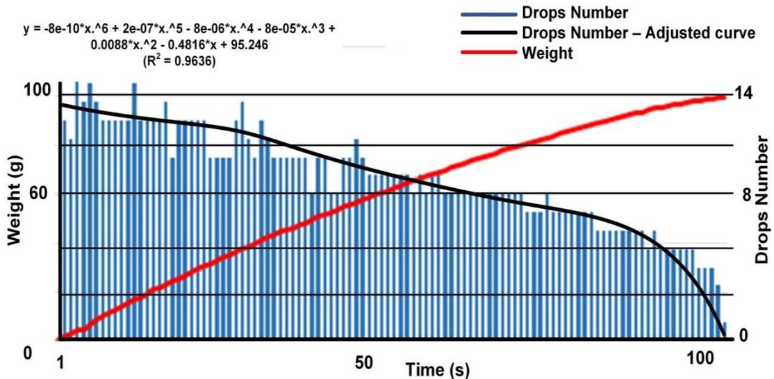
The experiment above was developed inside a laboratory with satisfactory results and it is important for scientific essays of irrigation system evaluation and characterization. However, its field deployment along a drip irrigation line requires the use of several computers on field, which can be a critical operation due to the computers physical size, high power consumption and risk of computers damage. Therefore, this work also
