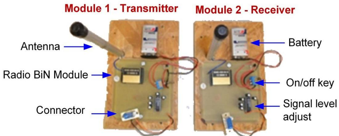
The module radio consumption for the data transmission operation is 17,5mA, which means that a battery type AA (length of 5cm and diameter of 1.45cm) with capacity of 2500mAh could supply this hardware for six days, while a motorcycle battery with 7Ah could provide power for seventeen days. Note that, it is for continuous daily transmission with batteries that can be rechargeable and besides the radio transmitter can also be
