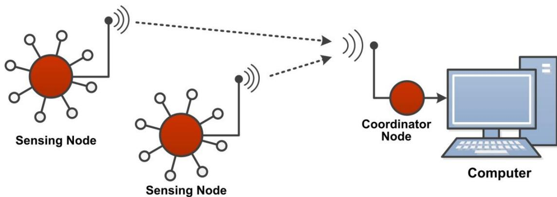
Figure 2 shows that each network sensing node was designed with sensors, a processing device and a radio
