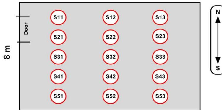
The work methodology was based on the temperature measurement in the greenhouse every fifteen minutes with an immediate data transmission for a computer where the data were recorded into a specific data base. This work includes the development of software to run on the Arduino board to perform de sensor data acquisition and its transmission, and another software to run on a personal computer, which receives the temperature
