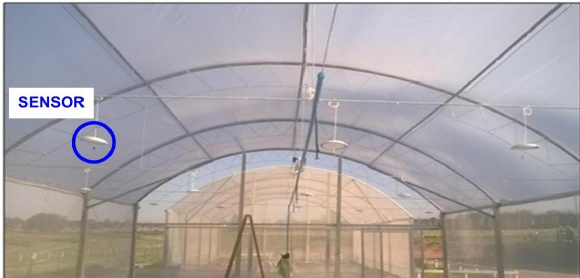
Figure 4 shows the mounted sensor structure, which was fixed under a plastic plate with an internal Styrofoam layer, which protected the sensor from the direct
