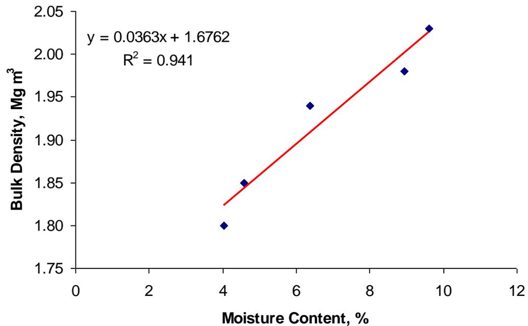
**Figure 1.** Soil compaction tests determination through the standard proctor tests.
