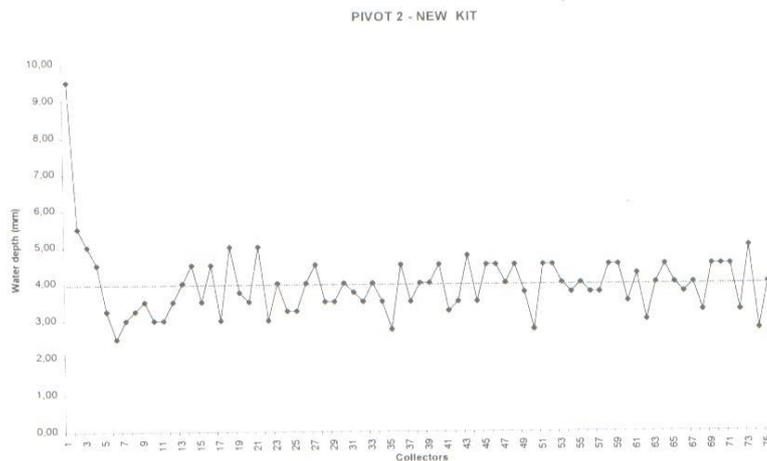
Fig. 4. Evaluation of water depth distribution for Pivot 2 with new pressure regulators and sprays.
