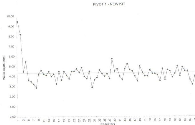
Fig. 3. Evaluation of water depth distribution with new sprays and regulators for pivot 1.
