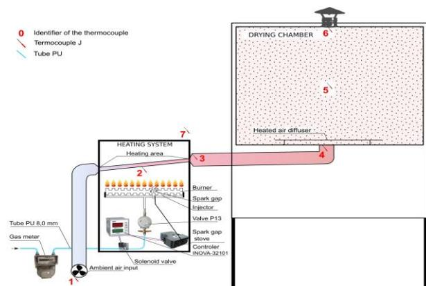
**Figure 1** - Diagram system of the heating and drying chamber with the provision of the temperature sensors (Thermocouples Type J)
